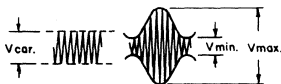
Fig.4 - The amplitude modulated wave; V_{car} is the amplitude of carrier before modulation.
